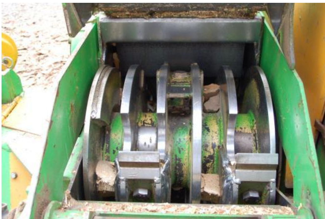
Figure 7 - Heizohack Chipper Showing Blades and 'Drum'
