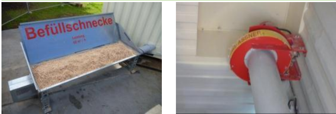
Figure 16 - Elevating Auger Showing Trough and 'Flicker' Head
