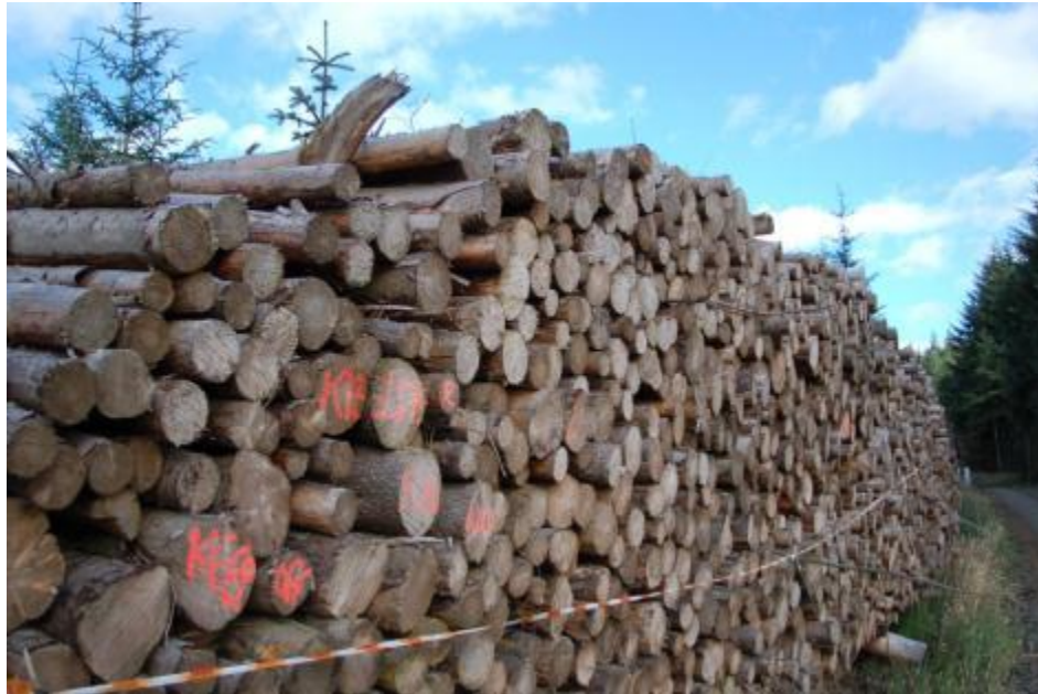
Figure 7 - Timber Stacked and Drying on Bearers
