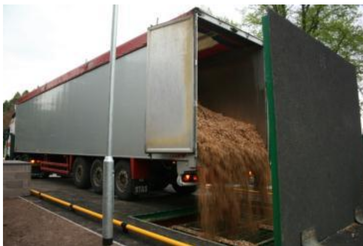
Figure 19 - Walking Floor Delivery (Image Taken : Crichton Hospital, Dumfries, 2009)
